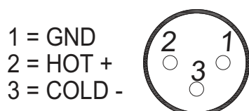
Fig2. XLR Bal Input / Output Pin-out
