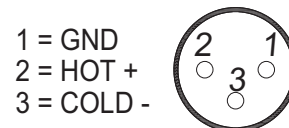
Fig1. XLR Bal Input / Output Pin-out
