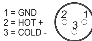
Fig1. XLR Bal Input / Output Pin-out
